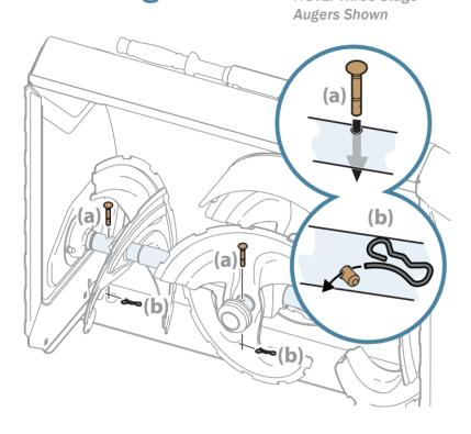
Shear pins are designed to break if the snow blower hits a hard object preventing damage to more expensive parts.
